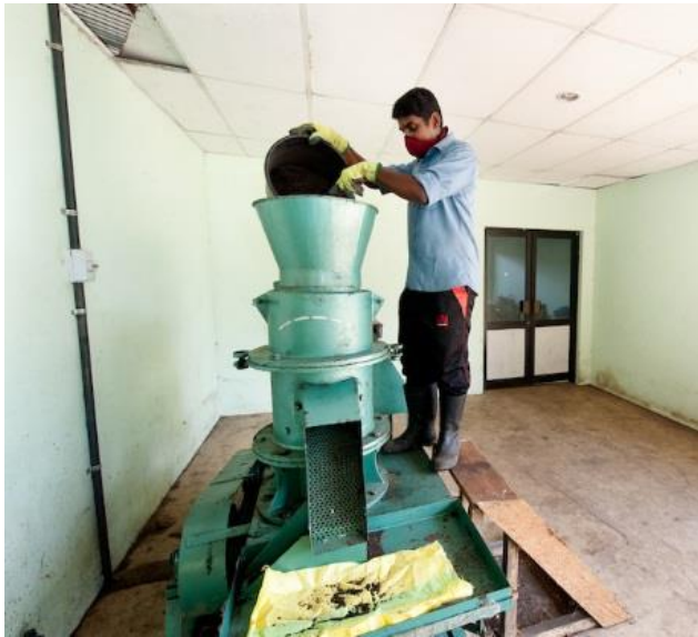
Figure 16: Feeding co-compost into the pelletizing machine
