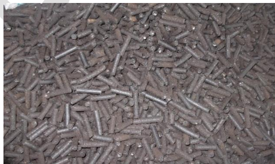
Figure 10 - Compost Pellets made with co-compost (MSW+ DFS) using die and roll pelletizer with 0-2.5 mm (PC1) particles and 25% moisture
